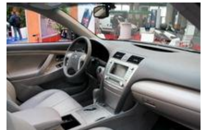
Toyota Camry Hybrid Interior - centre screen features the same graphic 'energy' display as the Prius
