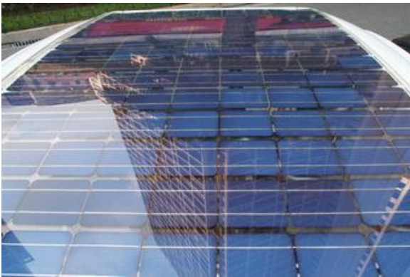
Venturi Eclectic solar roof, made up of multiple photovoltaic cells
