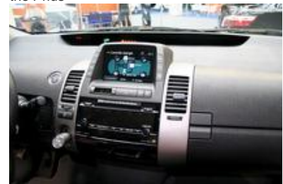
Prius interior characterised by the centre console screen displaying flows of energy in the hybrid drivetrain
